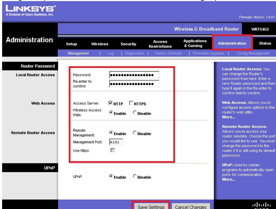
The screenshot shows the Linksys Administration interface for a Wireless-G Broadband Router (WRT54G2). The 'Administration' tab is selected. The 'Remote Router Access' section is highlighted with a red box. The settings are as follows:
